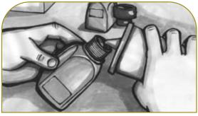
5. DIVIDING THE SAMPLE INTO THE "A" AND "B" BOTTLES
